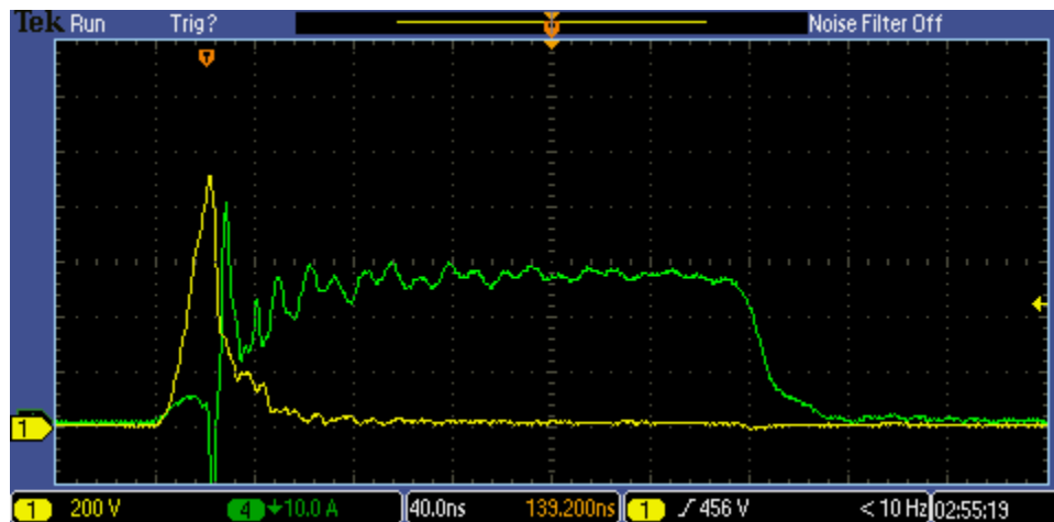
Figure 21. Load voltage (yellow) and current (green) for an arc and a 1 pF voltage divider.
