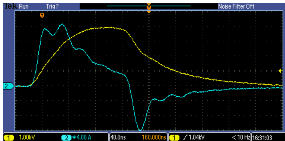
Figure 20. Load voltage (yellow) and current (blue) for a 35 pF DBD with a 5 k \Omega voltage divider.
