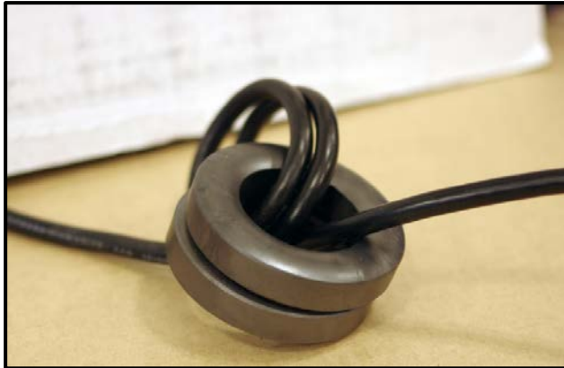
(Left) Cable wrapped loosely around two ferrites. (Right) Cable passed through a ferrite clamp.
