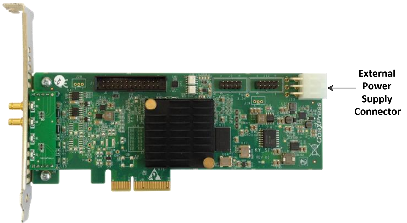
Figure 3: External Power supply connector
