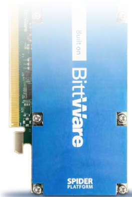
Spider Platform: designed for high-performance passive cooling in servers
