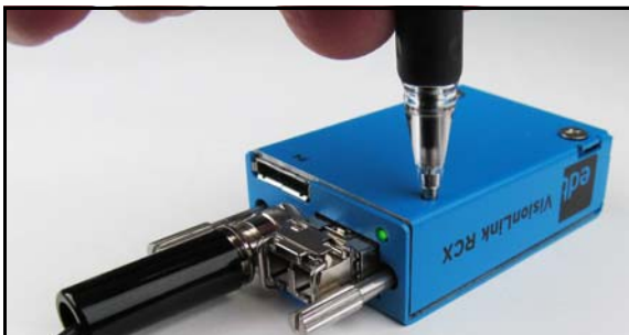
Figure 7. Pushing the recessed button
