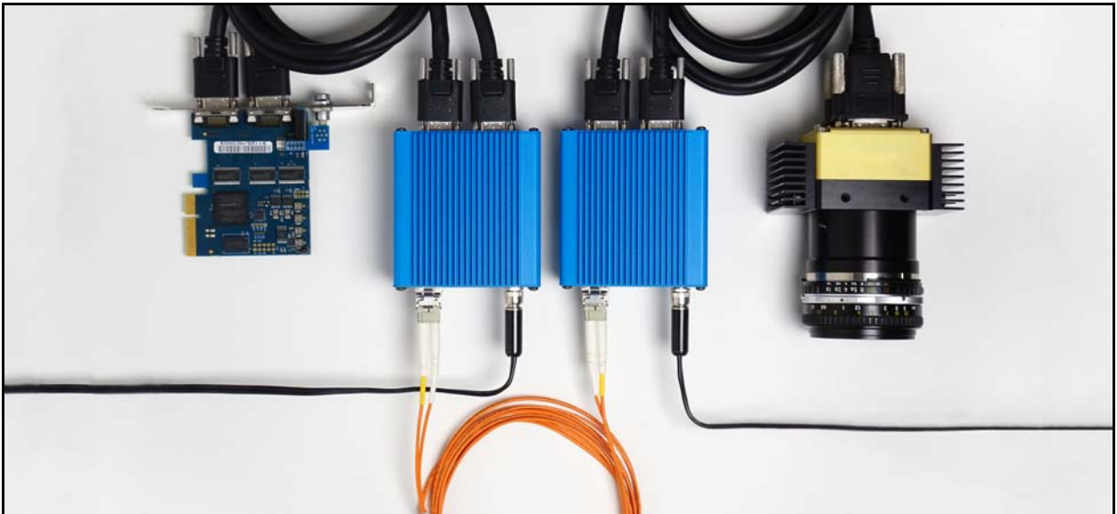
Figure 1. VisionLink XF extender pair – example setup (medium or 80-bit mode)
