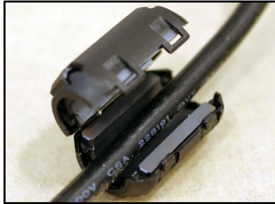
(Left) Cable wrapped loosely around two ferrites. (Right) Cable passed through a ferrite clamp.
