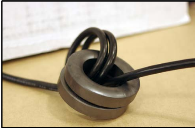
(Left) Cable wrapped loosely around two ferrites. (Right) Cable passed through a ferrite clamp.
