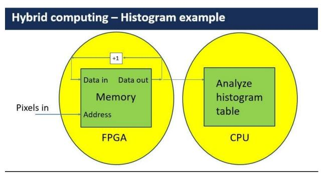
In a hybrid architecture, the FPGA handles repetitive number-crunching - incrementing pixel data - while the CPU analyzes the resulting histogram. Each processor does what it does best
