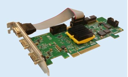
The Gidel HawkEye-CL frame grabbing and real-time image processing system provides the core infrastructure required to support the most demanding Vision and Imaging applications.
