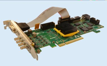
The Gidel HawkEye-CXP CoaXPress frame grabbing and real-time image processing system provides the core infrastructure required to realize the most demanding vision and imaging applications.
