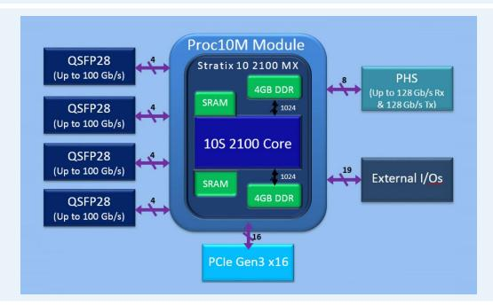
The off-the-shelf Proc1C carrier-board solution supports: PCIe Gen.3 x16 host interface, 4 x QSFP28 for up to 400 Gb/s aggregated bandwidth, Gidel PHS connector for mounting daughterboards, and 19 x GPIOs for peripheral system control. The PHS offers up to 128 Gb/s Rx/Tx enabling, for example, to connect 8x CoaXPress-12 \* cameras.
