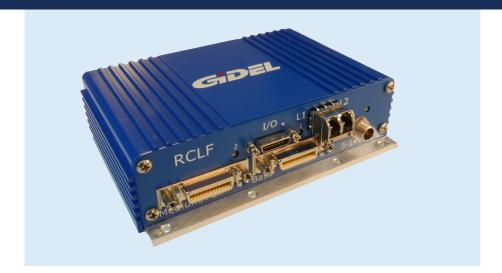
The Remote Camera Link Fiber-Optic (RCLF) extension system enables frame acquisition from a remote camera at a distance of up to 40 km without repeaters. A remote camera connects directly to the RCLF module that transmits the camera image over fiber optic cables to either a Gidel PCle HawkEye-CL frame grabber board mounted in a host computer or to another Gidel RCLGR module that can interface with any user frame grabber.
