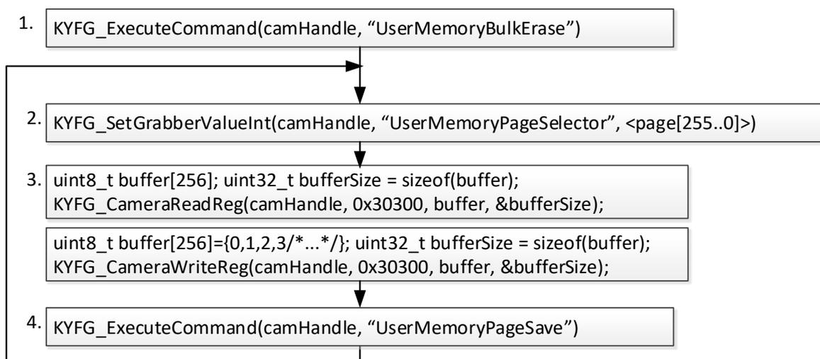
Figure 33 – Non-Volatile memory save function call sequence
