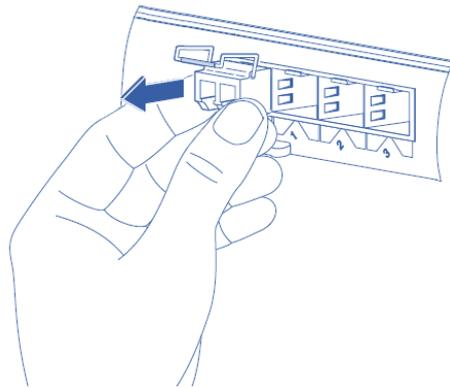
Figure 10 – Removing the SFP+ module from its port
