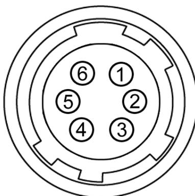
Figure 2 – GPIO connector pin out
