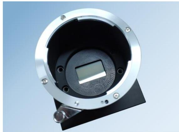
Figure 47 – Positioning the mount over the front panel
