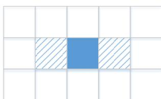
Figure 29 – Defect pixel correction position for Mono image
