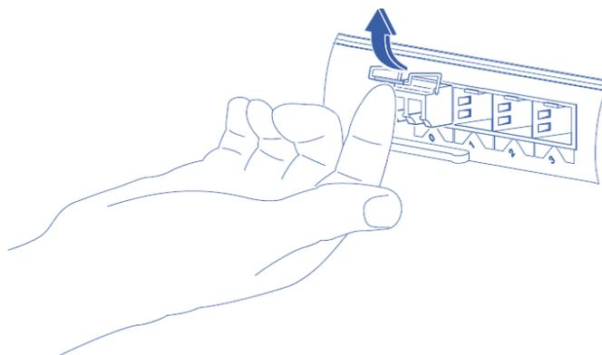
Figure 9 – Opening the bale clasp of an SFP+ Module
