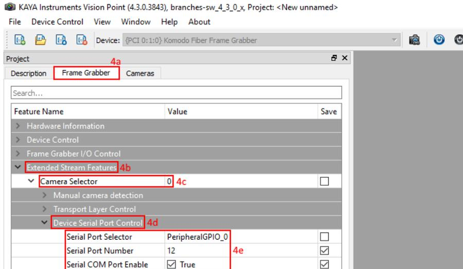
Figure 43 – Serial port setup at Frame Grabber side
