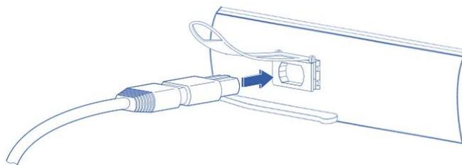
Figure 4 – Connecting the QSFP+ cable
