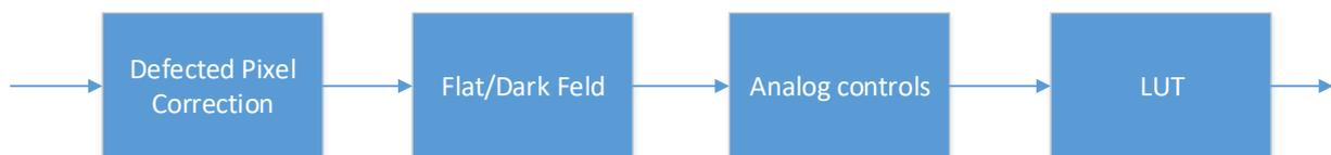
Figure 26 – ISP diagram flow
