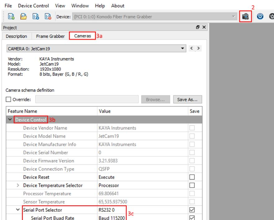
Figure 42 – Serial port setup at camera side
