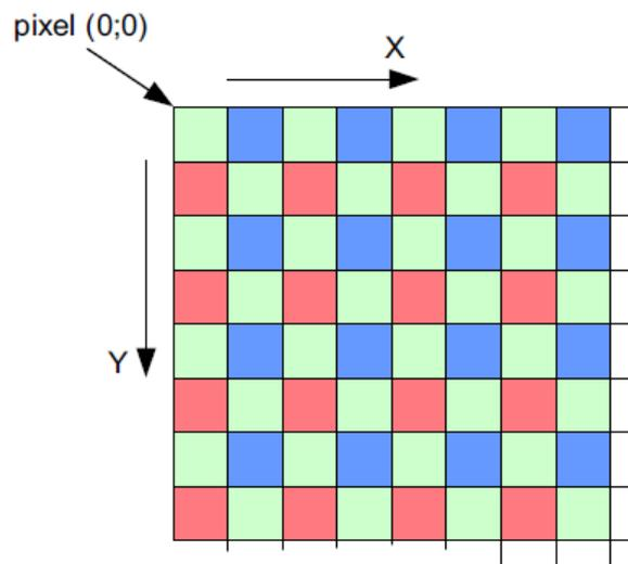
Figure 11 – Color Filter Array for the Pixel Array
