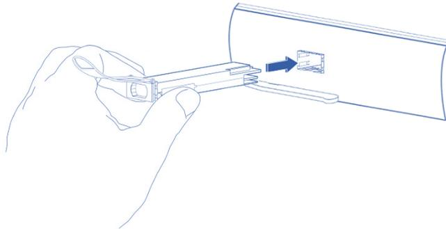
Figure 3 – Insert the QSFP+ module into the socket
