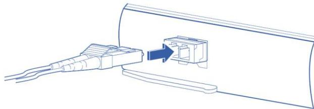
Figure 8 – Connecting the SFP+ cable
