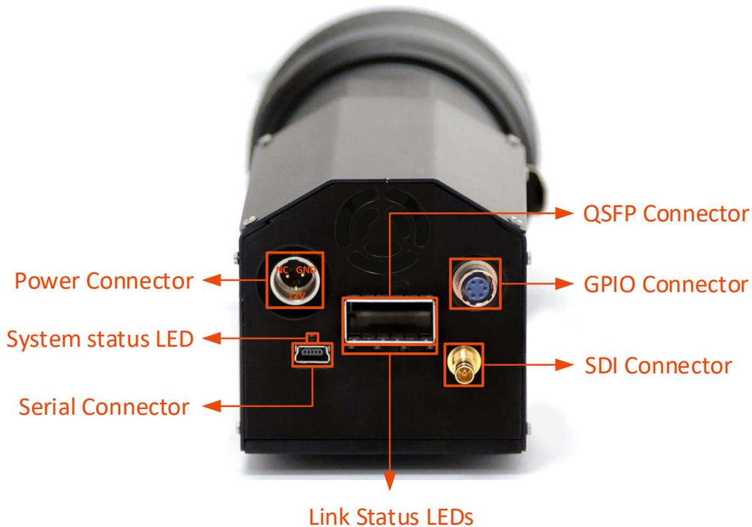
Figure 1 – JetCam camera interfaces
