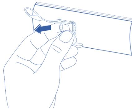
Figure 6 – Removing a QSFP+ Module from its port
