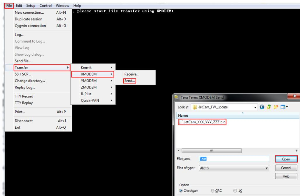
Figure 37 – Firmware terminal initiation
