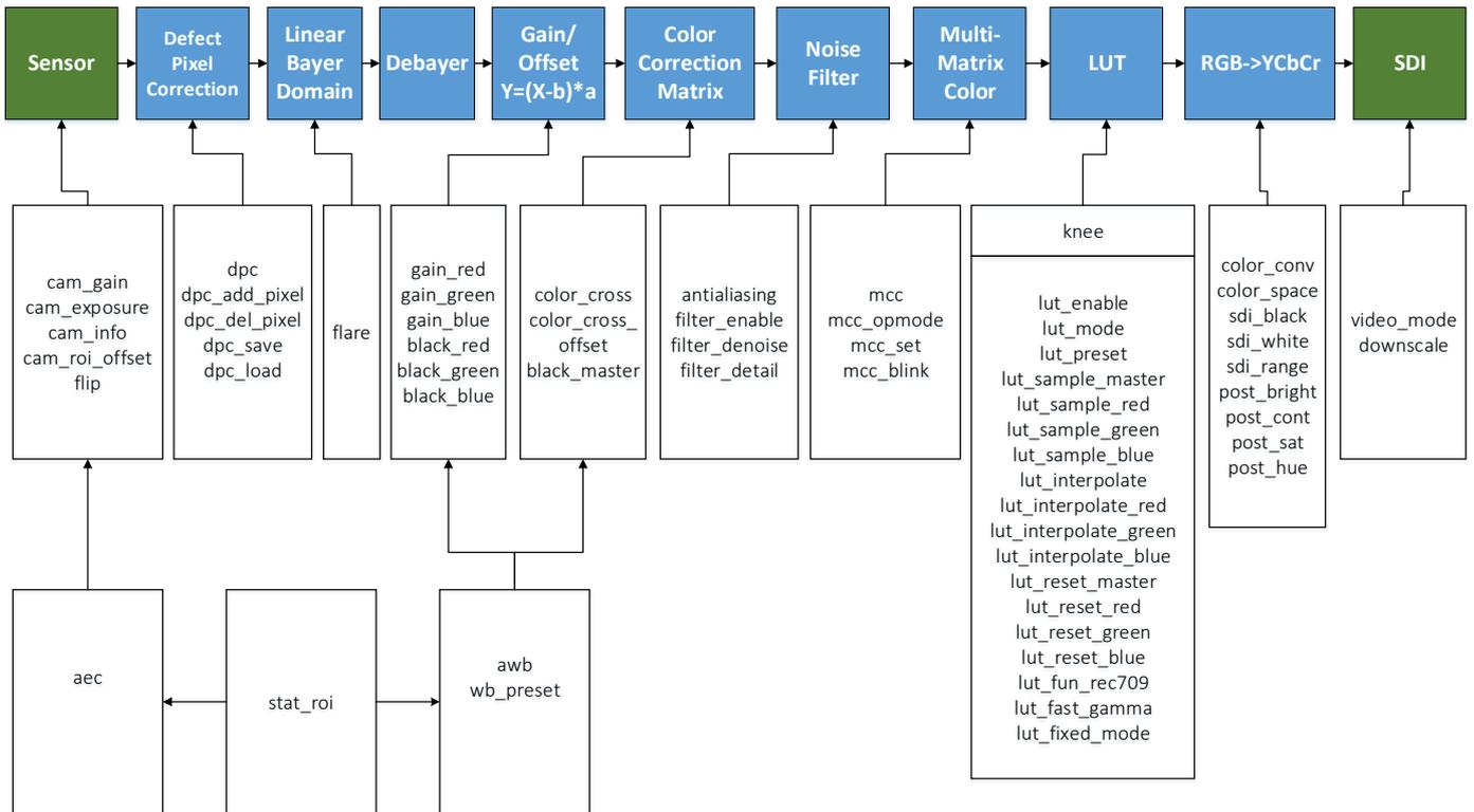
Figure 2 – Image Processing Flow
