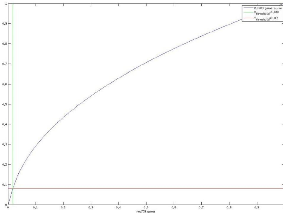
To avoid a discontinuity in the gamma-function select the brightness (offset) for the non-linear part by the following formula:
