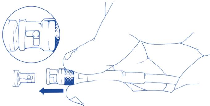
Figure 6 – Pushing the Micro-BNC connector into place
