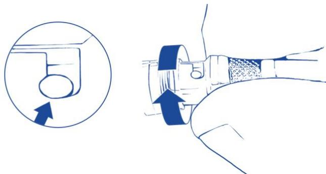
Figure 7 – Twisting the connector and securing it in position
