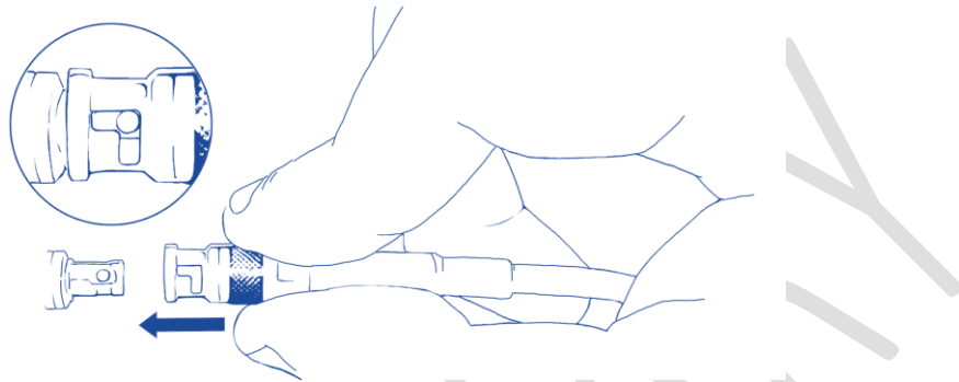
Figure 8 – Pushing the Micro-BNC connector into place
