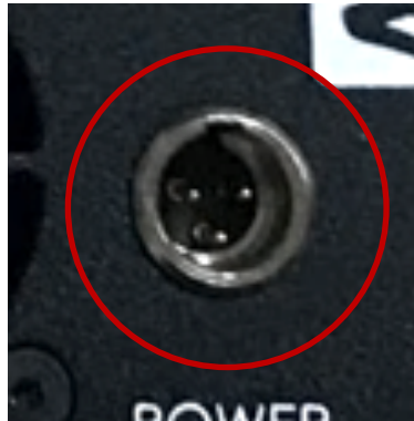
Figure 5 – KY-CL2F-D power connector
