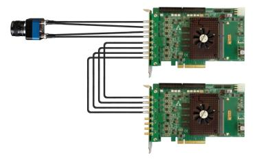
Figure 1: CoaXPress system block diagram
