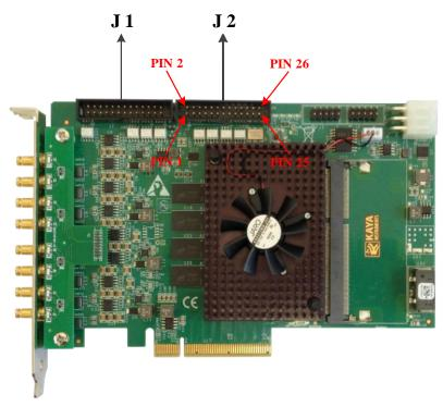
Figure 7: GPIO connectors location
