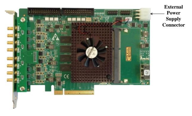
Figure 3: External Power supply connector
