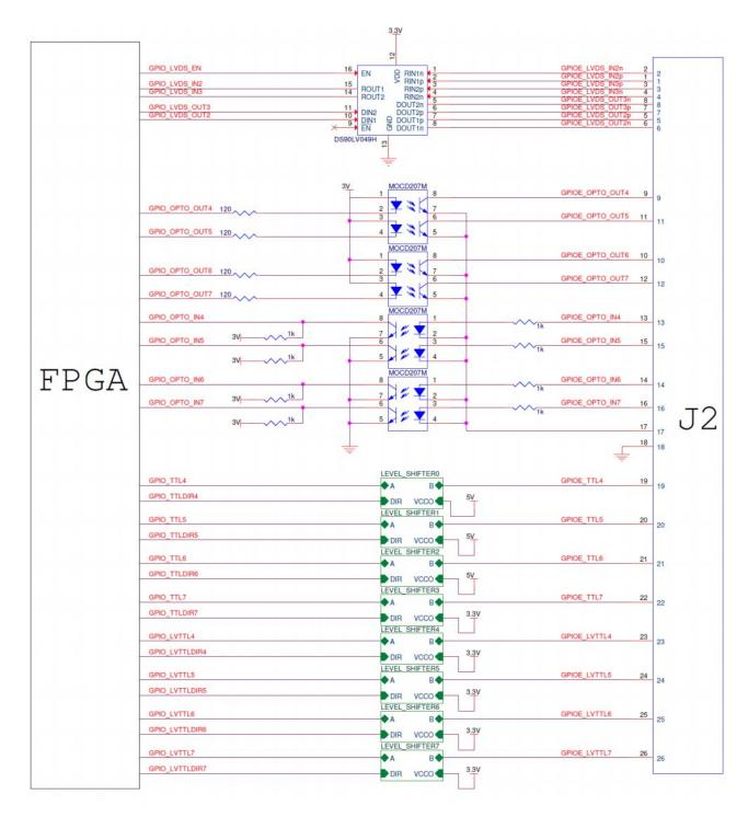
Figure 9: J2 general purpose inputs and outputs connectors schematics
