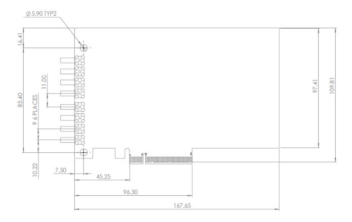
Figure 4: PCB Mechanical Dimensions
