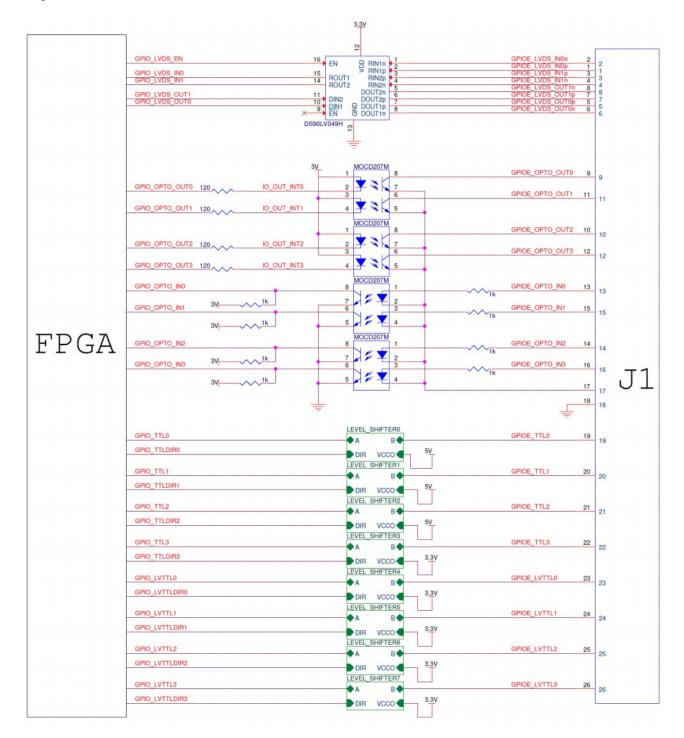
Figure 8: J1 general purpose inputs and outputs connectors schematics
