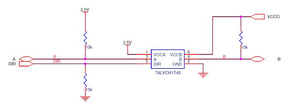
Figure 10: Level shifter schematics
