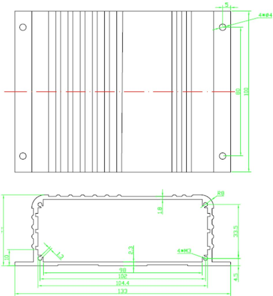
Figure 16 : External dimensions of the KY-EXT-CL enclosure box
