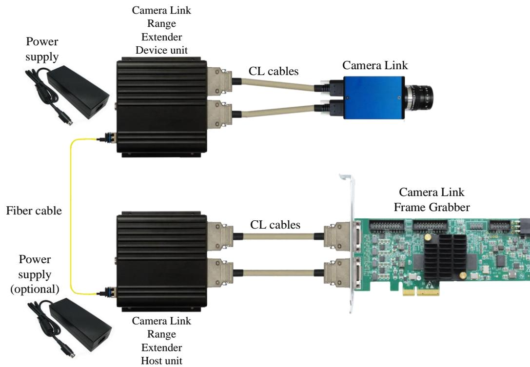
Figure 12 : Bidirectional Camera link connection
