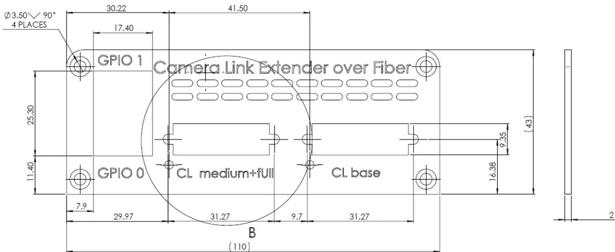
Figure 14 : External dimensions of the KY-EXT-CL Camera Link side panel
