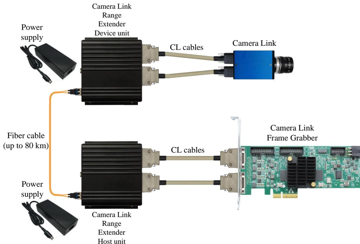
Figure 3 : KY-EXT-CL connection diagram
