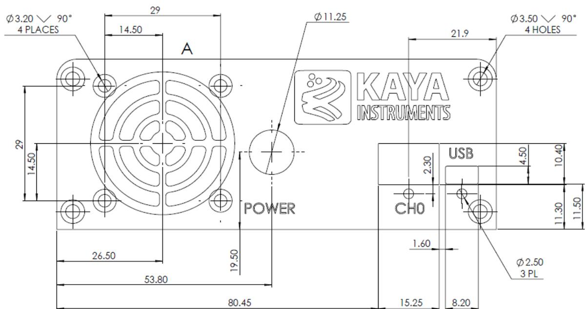
Figure 15 : External dimensions of the KY-EXT-CL Fiber side panel
