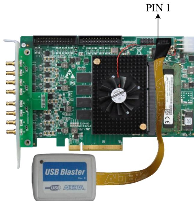
Figure 1 : Komodo Frame Grabber board with USB-Blaster™ attached
