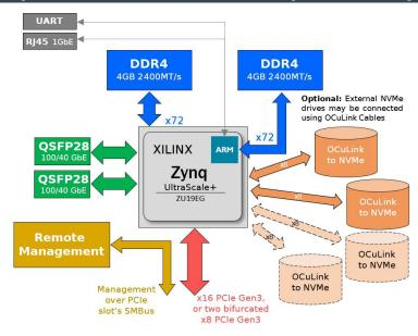
» SMBus access to unique board data and temperature sensor
