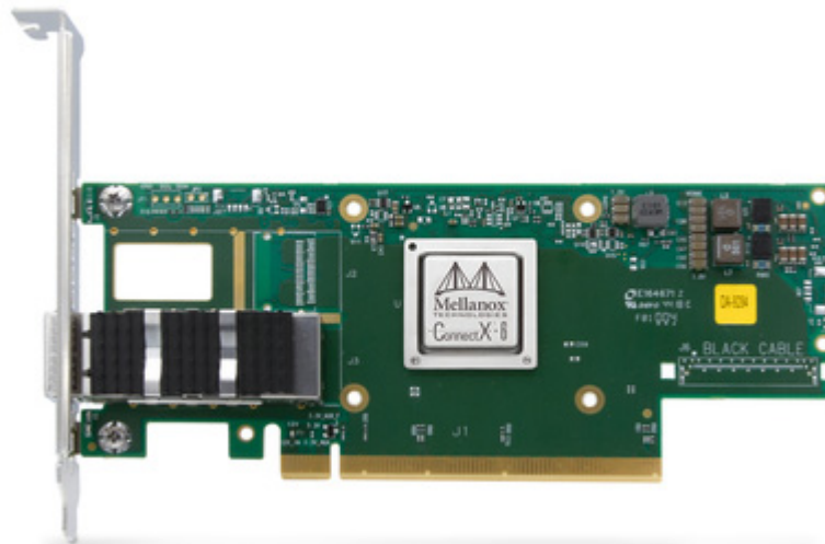
Figure 10. Mellanox Single-port ConnectX-6 VPI card for highest network throughput
