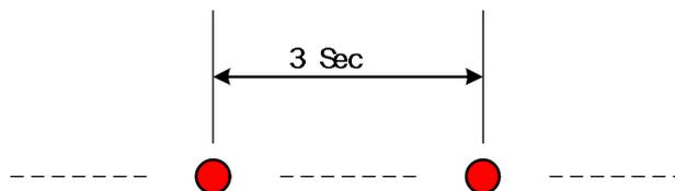
▶ Optical line is not connected.
